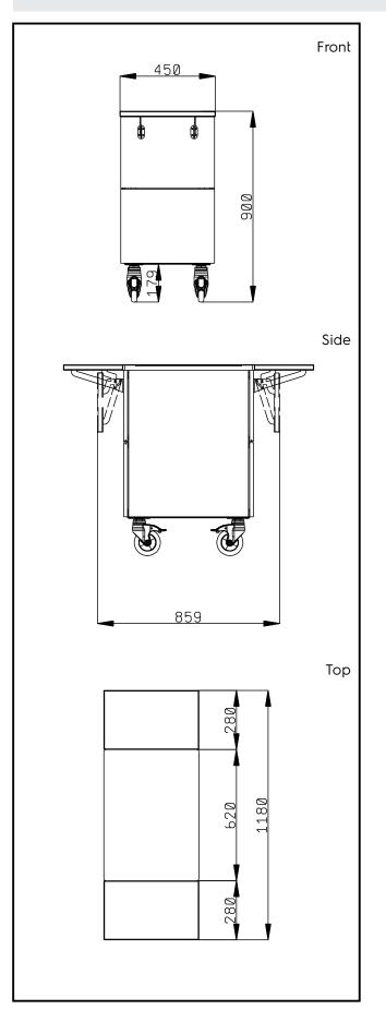
Flexy Compact Ambient unit on cupboard (IGN) with wheels, overshelf with LED lights, H=900mm The company reserves the right to make modifications to the products without prior notice. All information correct at time of printing.
